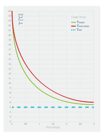
However, this is only half the story of the Quest II system. In traditional chilled reefers the evaporator fans are always set at maximum speed, but Quest II is programmed to adjust the internal air circulation according to the actual cargo heat load.
